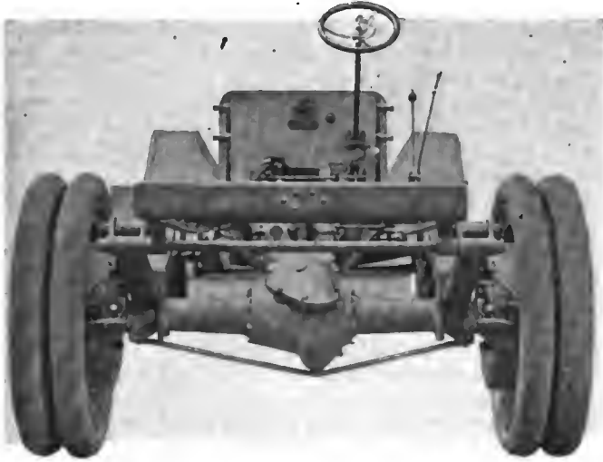
Rear Construction and Twin Tires on White Gasoline Truck
